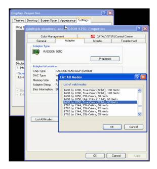
Note: If your video/ graphic card does not support the resolution of 1680 x 1050, then you can try to set the resolution to 1280 x 960 or 1280 x 768 to avoid picture stretching.
